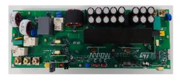
Advantages: Approx. 50% reduction in size vs IGBT design, High output power (6.6kW Max.), High efficiency (>98%), Digital control bidirectional output, Reinforced isolation, Workable firmware ready.
